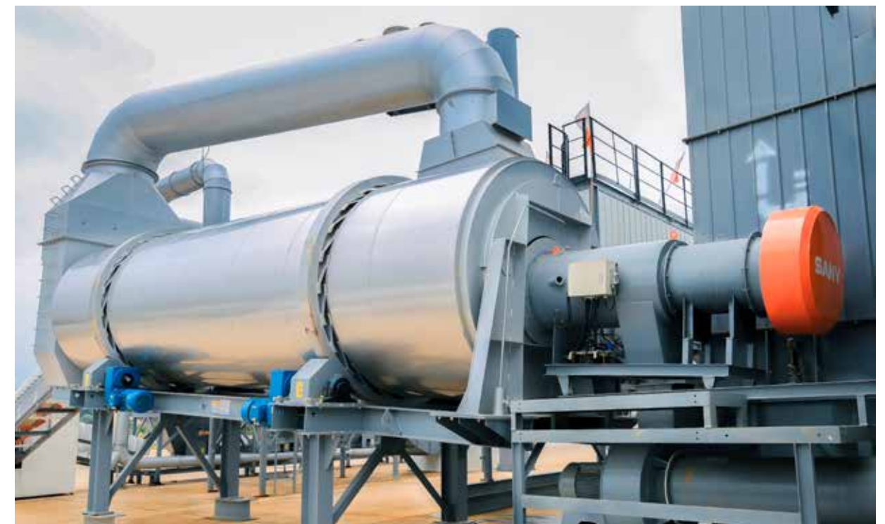
● 烘干滚筒 Drying roller
