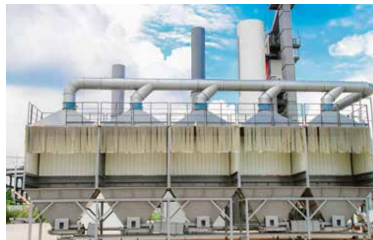
● 上料系统：冷料防尘罩效果图 Effect Picture of Cold Aggregate Dust Shed and Cover for Feeding System
