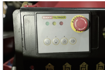
Overload Protection System
